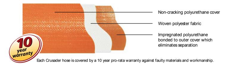
The woven polyester fabric jacket gives the hose its high bursting and tensile load features. The polyurethane cover not only protects the hose against abrasion damage but also against harmful UV radiation and ozone. This unique design renders the hose lightweight yet extremely strong and durable.
