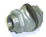
**CAUTION:** Use only Nickel Plated or Plastic Ball Valves & Tank taps with Zinc Alloy Fittings. **Brass Gate valves cause the fittings to corrode due to electrolysis.**
