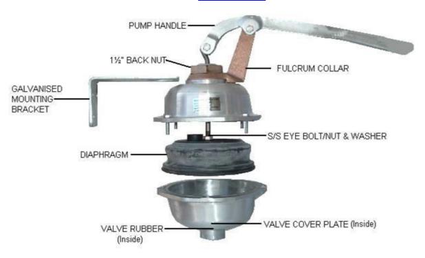
This "Read Hand Priming Pump" has a heavy duty polished Aluminium body with an Aluminium fulcrum collar. The Diaphragm is very solid rubber with a metal plate encompassed in the bottom for extra strength. Each Stroke displaces 1.9 litres of Air.
