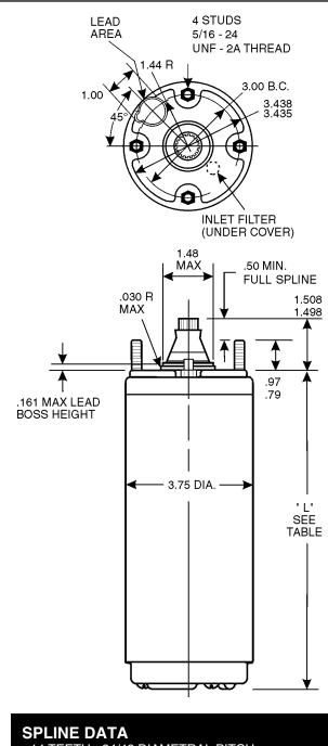
• 14 TEETH • 24/48 DIAMETRAL PITCH • 30° PRESSURE ANGLE • FLAT ROOT, SIDE FIT SLIDING CLASS "A" FIT • ASA B5.15-1950
