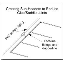
• To reduce the number of glue joints, saddles or insert fittings in a header, transition to Techline and Techline fittings to make up sub-headers, making sure to follow the guideline of a maximum of 5 GPM in the "sub-header" zone.
