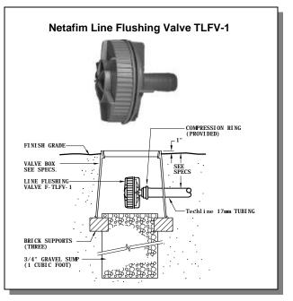
Line Flushing Valves should be buried in
