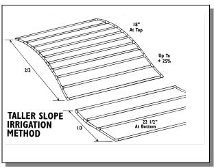
usually have a slope of 1% to 4%. In these cases you may wish to use inline check valves to prevent drainage of the water inside the piping network to the lower elevations.
