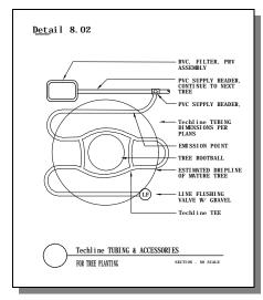
• A loop of Techline close to the rootball, with more Techline surrounding the estimated drip line of the tree when mature will provide sufficient water. *SEE Detail 8.02.*
