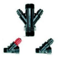
If zones are designed to flow between 3.5 GPM and 20 GPM, use the PRV075**HF**15, 25, or 45. The difference in which regulator to use refers to which Techlite dripperline is being used. If Techline is being used, it is usually easiest to use a 45 PSI regulator.
