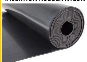
Black natural insertion rubber nylon reinforced, is a black, superior grade, 60 Duro blended natural synthetic rubber sheet, reinforced with a tear resistant nylon monofilament fabric. The specially designed nylon monofilament fabric reinforcement will not allow fluid penetration and gives natural insertion improved tear strength and dimensional stability, making natural insertion specifically suitable for gasket sealing applications.
