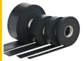
Black natural insertion rubber 60 Duro blended natural and synthetic rubber strip, reinforced with cotton fabric for improved tear resistance and dimensional stability. Available in standard widths or custom on request. Good physical properties such as mechanical strength and tear strength and has moderate abrasion resistance making it suitable for general insulating or isolating and gasket sealing applications, as a flexible strip, pad,
