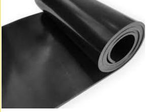
Neoprene 60 rubber sheet is a black, superior grade 60 Duro blended neoprene and synthetic rubber sheet. Good mechanical strength and is flexible and resilient with moderate temperature and flame resistance. It has some petroleum based fuel and oil resistance. Neoprene 60 rubber is UV stable and is resistant to ozone effects and weathering. Ideal to use as a flexible strip, pad, lining or gasket. Primarily designed to seal, protect, insulate & isolate.
