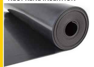
Neoprene insertion rubber is a black, superior grade, 60 Duro blended neoprene and synthetic rubber sheet, reinforced with tear resistant nylon monofilament fabric. It has good mechanical strength and is flexible and resilient with moderate temperature and flame resistance. It has some petroleum based fuel and oil resistance. Suitable for gasket sealing applications, UV stabilized & resistant to ozone effects and weathering.
