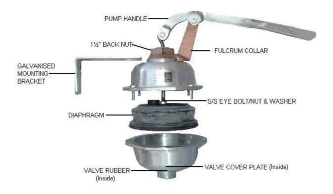
This "Read Hand Priming Pump" has a heavy duty polished Aluminium body with an Aluminium fulcrum collar. The Diaphragm is very solid rubber with a metal plate encompassed in the bottom for extra strength. Each Stroke displaces 1.9 litres of Air.
